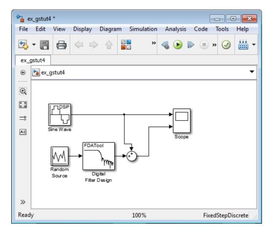
**3** Run your model and view the results in the Scope window. This window shows the original input signal and the signal with low frequency noise added to it.
